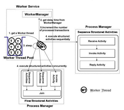
Figure 9. Worker threads for executing complex structured activities.
