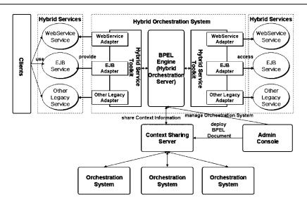
Figure 6. Software architecture of the orchestration system.
