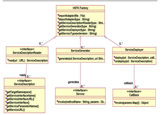
Figure 7. Design of the hybrid service toolkit.
