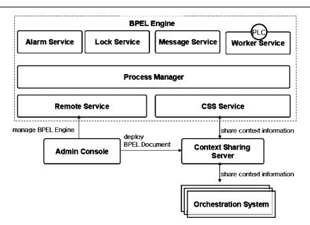
Figure 8. Software architecture of the BPEL engine.
